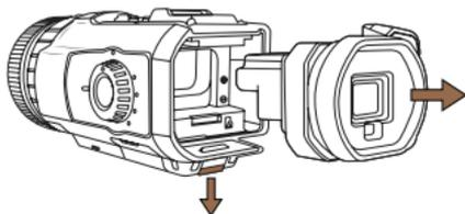
2. Install battery and Micro SD card
